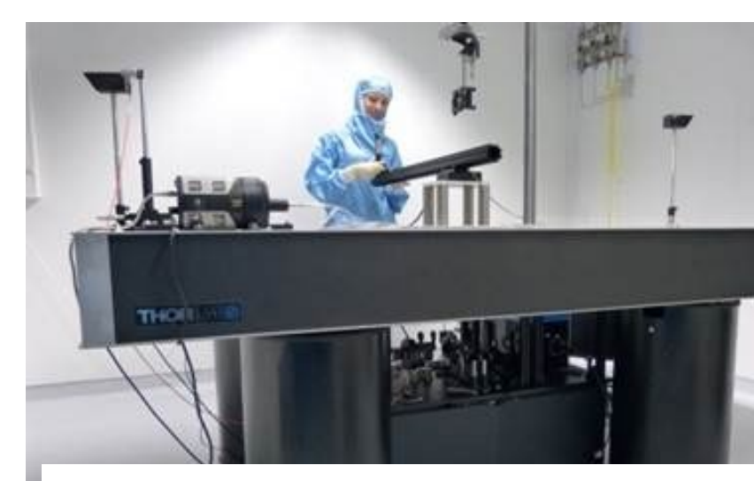
Diffusion Spectrale SALSA - Spectral and Angular Light Scattering characterization Apparatus
